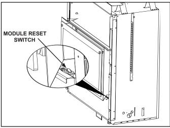
Figure 2.5 Location of Module Reset Switch - Martini Front
